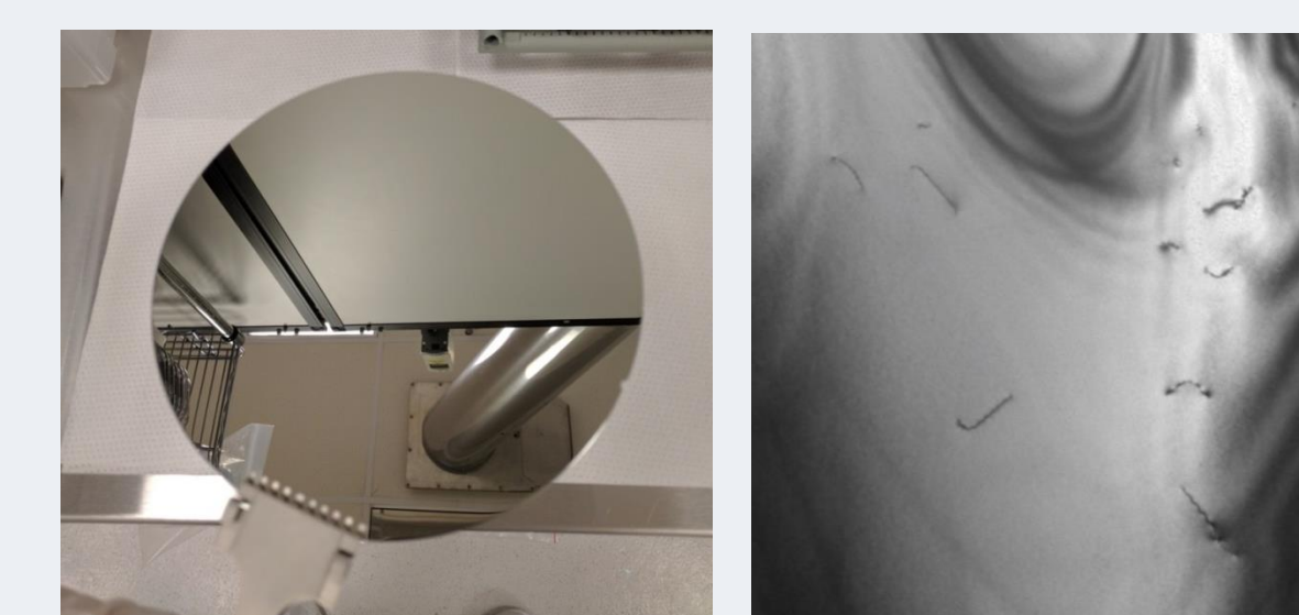
Specular Ge film surface and TEM image of threading dislocations in Ge on Si system
